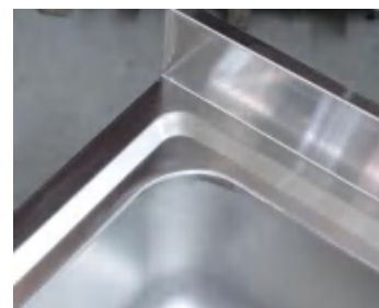
Nice polishing finish after welding
